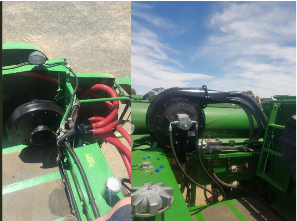
Smal aire blower kit fitted to John Deere Headers
