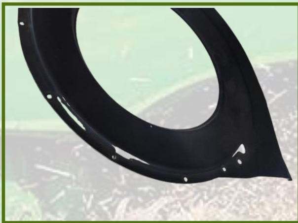
Pictured above is the new Stainless Steel halves installed after the plastic halves have worn out.
