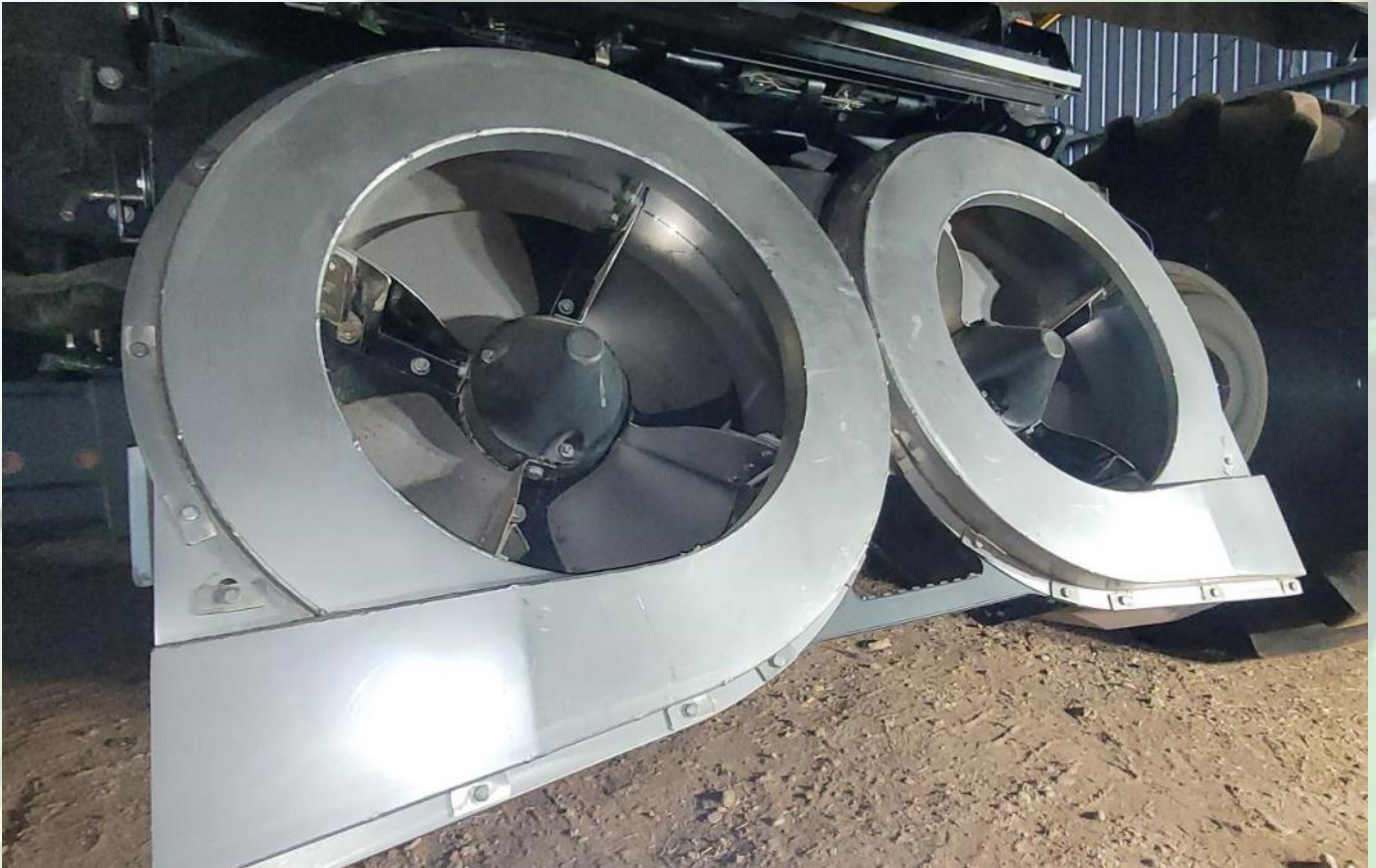
Pictured above is the new Stainless Steel halves installed after the plastic halves have worn out.
