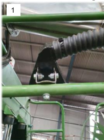
Pictured above is the Smallaire Blower Kit installed on a 8 string Baler.
