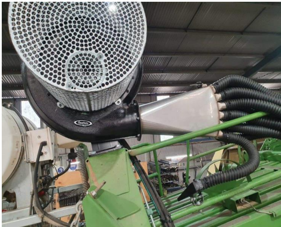
Pictured above is the Smallaire Blower Kit installed on a 8 string Baler.
